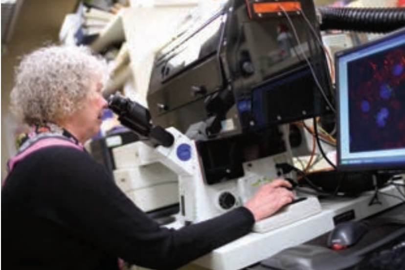
Kane uses confocal fluorescence microscopy to visualize uptake of carbon nanotubes by target cells.
